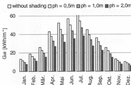
Figure 5: Seasonal variation of the diffuse radiation with and without overhang.
