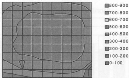
Physical model studies and computer simulations predicted adequate illumination levels in the gallery and offices. Under low daylight levels, supplemental electric illumination will be required.
