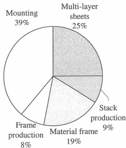
Figure 9: Cost split of the sheet TI system.
