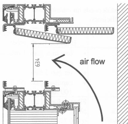
*Figure 3: Vertical section of upper ventilation opening with double flaps (no gear included).*
