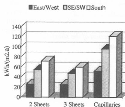
Figure 2: Energy gains per m<sup>2</sup> solar wall heating.
