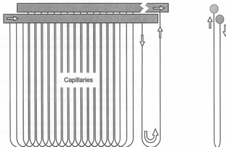
Figure 2: Principle of capillary piping.
