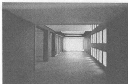
A physical model of the same space produces accurate illumination and a visual realism with sufficient detail. All three tools can help designers make appropriate decisions.
