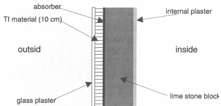
U-value of the opaque wall:  $U_W = 1.26 \text{ W/m}^2\text{K}$
