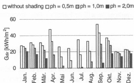
Figure 4: Seasonal variation of the direct radiation with and without overhang.
