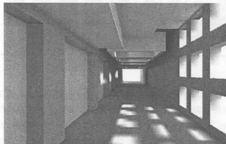
The Lumen Micro program produces grey-scale renderings and luminance readings at any point in the image. This image shows the gallery daylighting at 10:00 on a clear December day.
