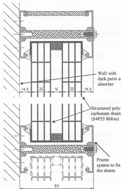
Figure 4: Vertical section of the sheet TI system.
