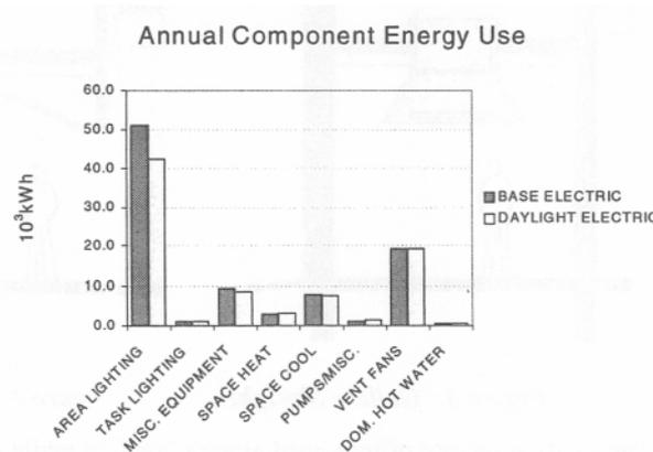
The VisualDOE analysis predicted the energy savings potential of a properly design daylighting retrofit. In this case, a slight increase in the heating and cooling loads was more than offset by electrical energy savings.
