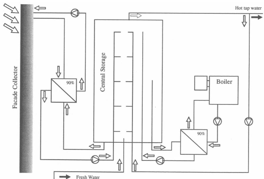
Figure 3: Basic system layout for the simulation.
