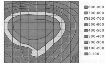
The graphs of the lux levels in the office predict uniform illumination with daylighting in December versus excessive illumination with the existing electric lighting.
