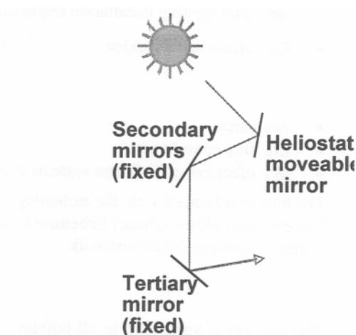
Figure 1: Light guiding principle with Heliostat mirror.
