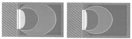
*Figure 6: The daylight distribution before and after the adding of the glazed balcony (left before, right after renovation; contour levels see figure 7).*
