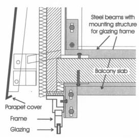
The existing balcony structure was insufficient to bear the additional wind load of the new glazing. Thus, a steel reinforcement was necessary to anchor the glazing frame on facade.
