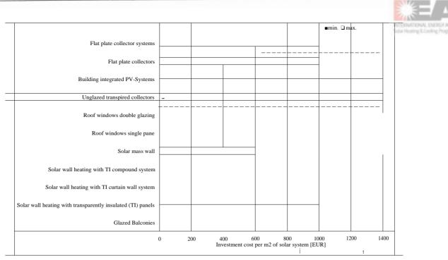
*Figure 3-1: Investment cost of solar renovation concepts found under Subtask A (in C/m2 solar system)*
