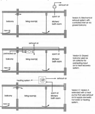
Figure 1: Principles of the different ventilation concepts.
