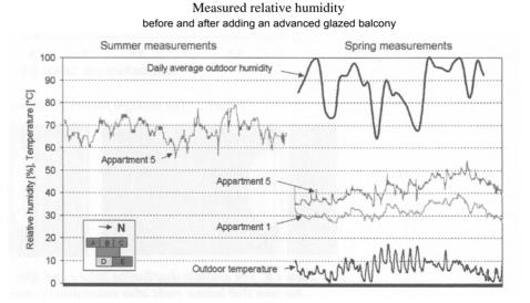
Figure 3: Measured humidity levels in apartments before and after renovation in apartment A and D (see corresponding floor plan of figure 2).
