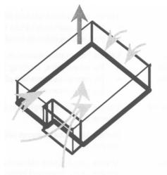
Figure 1: Schematic of the airflow through the apartment: intake by vents in the walls and the balcony and the extraction by a central exhaust system.
