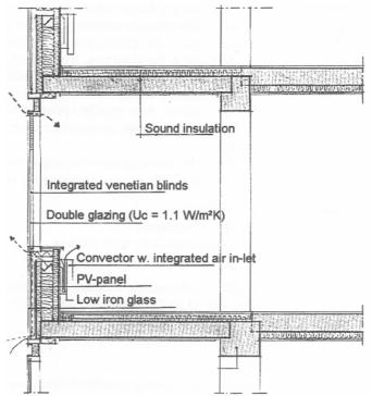
*Figure 1: Vertical cross section of advanced glazed balcony.*
