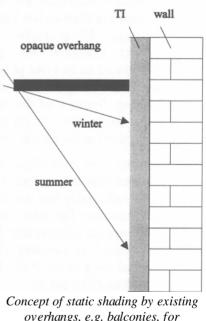
overhangs, e.g. balconies, for seasonal gain control of solar wall heating systems.
