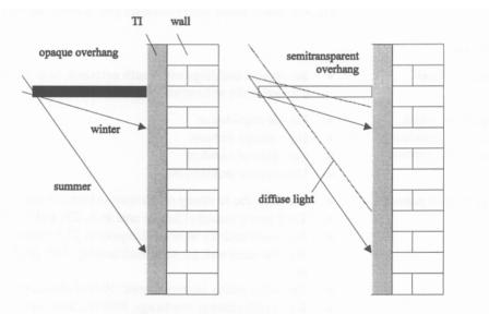
Figure 1: Principle of static shading by an overhang.Left: opaque overhangRight: selective overhang
