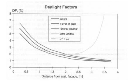
Figure 5: The daylight factors for different glazings.
