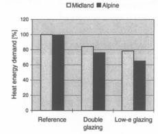
Figure 5: Heat energy reduction in function of climate (reference refers to double-glazing and no air preheating).
