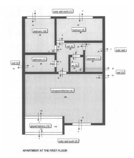
Figure 3: A ir distribution with **high** air flow input through balcony (figures in brackets are room numbers in the simulation model)
