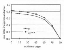
Figure 7: Transmission characteristics selective absorber.
