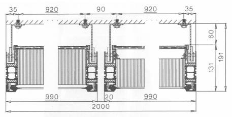
Figure 2: Horizontal section of the two prototype constructions: high inertia absorber on the left, selective surface absorber on the right.
