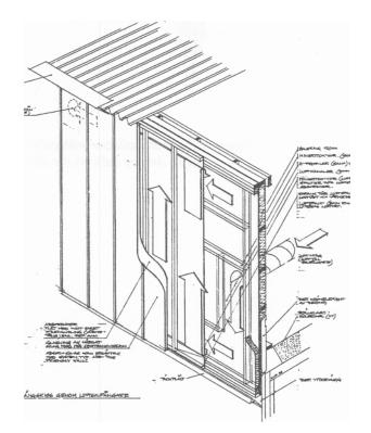
Figure 2: The reproduction of the blueprint shows the planned airflow of the west facade in 3-d view. Courtesy of C. Nordstrom.
