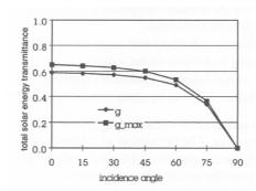
Figure 6: Transmission characteristics high inertia absorber.
