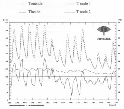
Figure 4: Temperature curve in construction, summer (1 Jul. – 15 Jul.); position of temperature nodes see figure 3.
