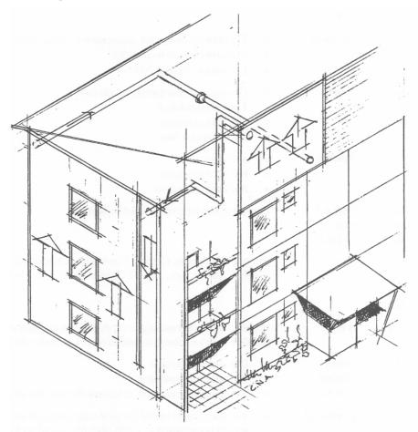
Figure 1: The illustration shows a schematic drawing of the solar air system with double envelope. Courtesy of C. Nordström.
