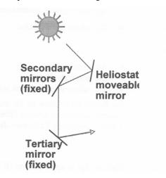
Figure 1: Light guiding principle with Heliostat mirror.
