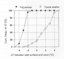
Figure 8: Cumulative frequency of the temperature difference between inner wall surface and room air for a wall with an equivalent U-value of  $0.5 W/(m^2.K)$  and the solar wall prototype.
