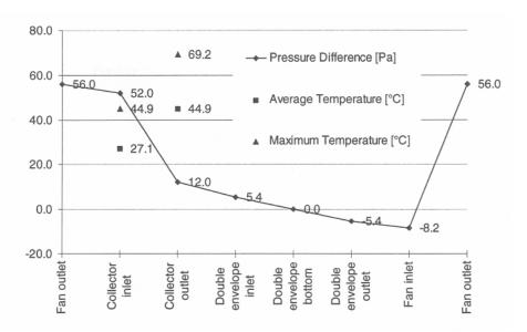
*Figure 8: Pressure profile in Pa and average temperatures in °C of a typical system while fan is feeding the collector.*
