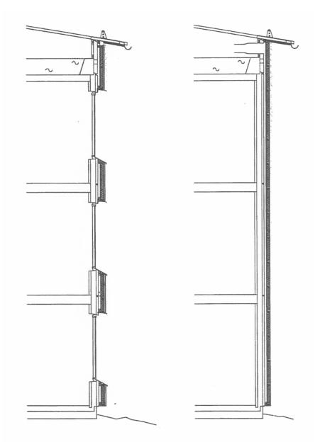
Figure 4: Double envelope: Facade part with windows (left) and closed facade part (right). Courtesy of C. Nordström.
