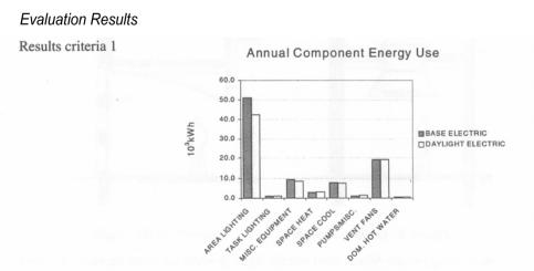
The VisualDOE analysis predicted the energy savings potential of a properly design daylighting retrofit. In this case, a slight increase in the heating and cooling loads was more than offset by electrical energy savings.
