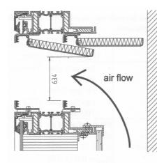
Figure 3: Vertical section of upper ventilation opening with double flaps (no gear included).
