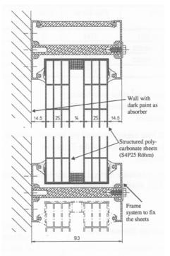
Figure 4: Vertical section of the sheet TI system.
