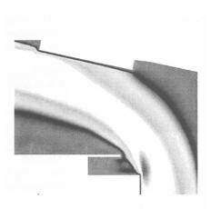
Figure 4: Simulated air flow pattern of upper ventilation opening: laminar air flow (light grey) with turbulent zones (dark shades) and static areas (dark grey)
