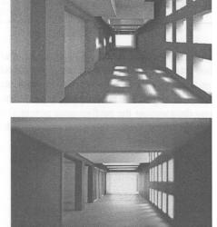
A physical model of the same space produces accurate illumination and a visual realism with sufficient detail. All three tools can help designers make appropriate decisions.
